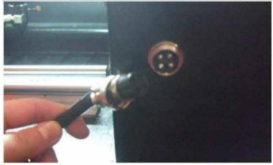
2) then plug the wire in the port to connect the machine:
